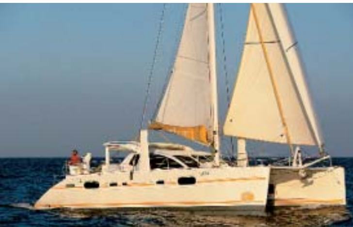
Daggerboards are essential equipment for high-performance catamarans; note also the asymmetric hulls on this Catana
