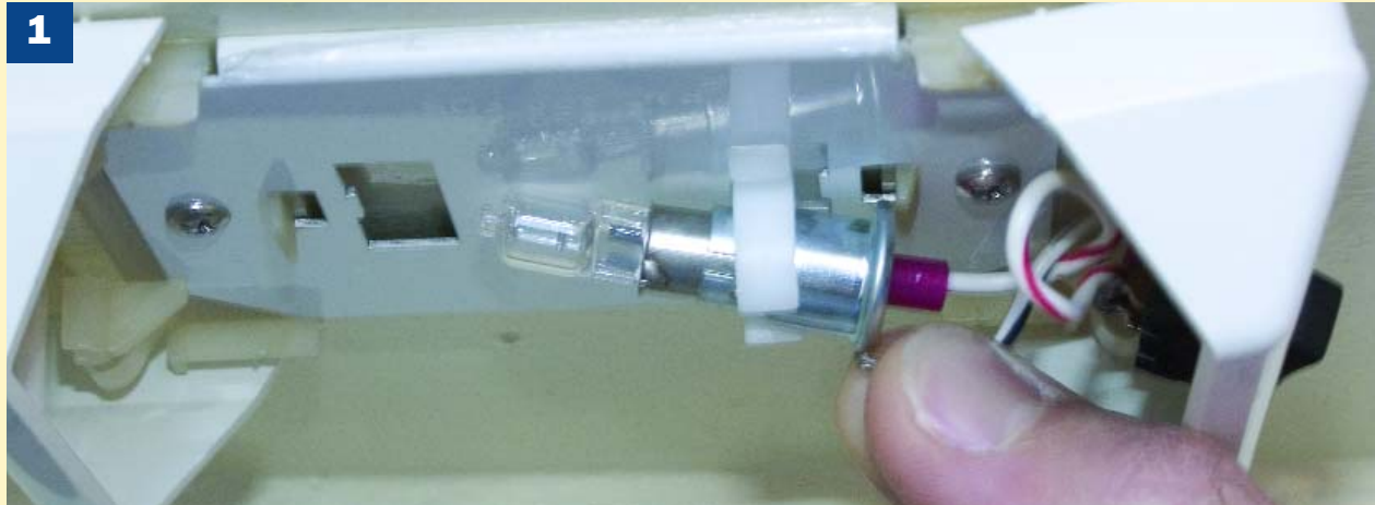
1. Remove the cover of the light and pull out the existing bulb, noting which wire is the positive (normally red) and which is the ground (normally black).
