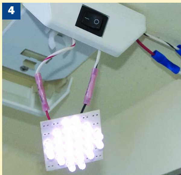
4. Make sure the wires are connected the right way round before you crimp the wires to the lighting fixture.
